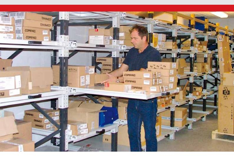
Upright-mounted (UM) units are hung directly from the pallet racking uprights, rather than being supported by a cross-beam. The lower frame of the unit is bolted to the uprights and the upper carriage slides out, carrying the load with it.
