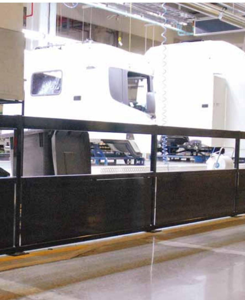
We make two types of workplace protection systems. **Safety rails** separate personnel from machinery and other dangers and demarcate safe walkways. They are also useful where there is a sudden change of level, such as around mezzanine floors. **Safety barriers** offer much more solid protection, especially against fork-lift trucks and other vehicles, in any area where people and vehicles have to share the same space.
